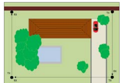
Solution with terminal and bi-directional barriers
