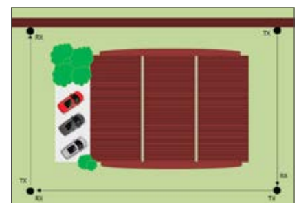
Solution with terminal and bi-directional barriers
